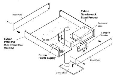
Figure 2-7 — PMK 350 projector mounting a receiver
